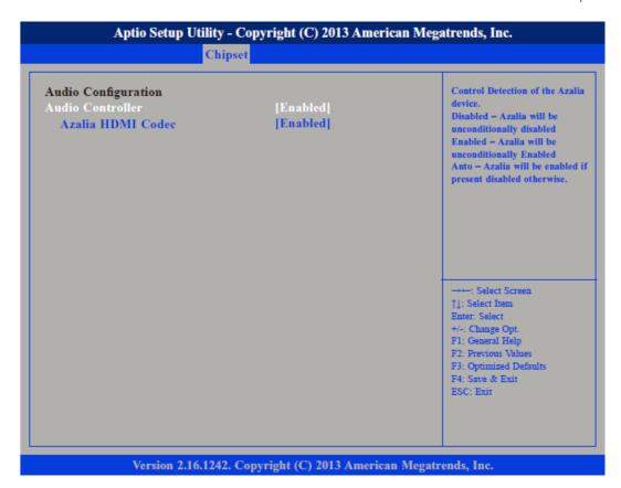
Audio Controller Control detection of the Azalia device.
