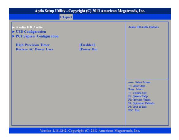
**High Precision Timer** This section is used to configure *High Precision Event Timer*.
