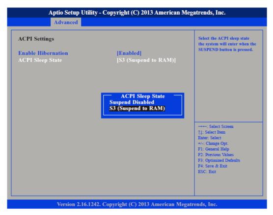
Select the highest ACPI Sleep State the system will enter when the suspend button is pressed.
