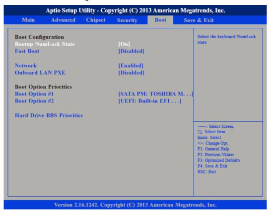
Bootup NumLock State This allows you to determine the default state of the numeric keypad.
